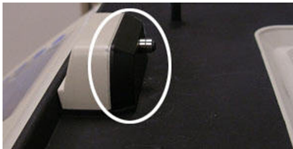
Figure 86. Optical module locking latch.
