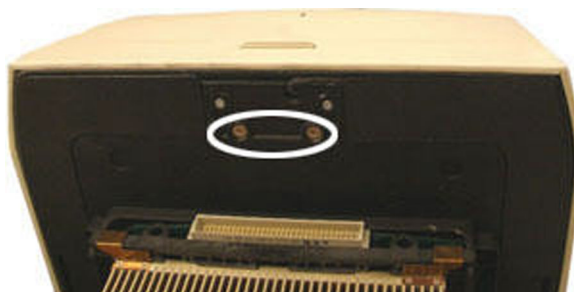
Figure 85. Remove these screws to unlock the optical module.
